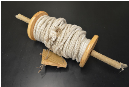
The chip log measured the ship's speed in knots
